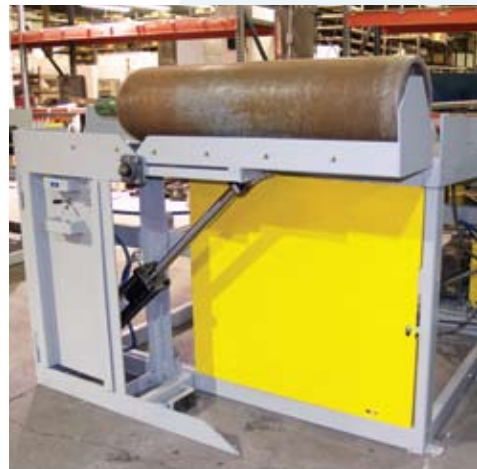
Pneumatically controlled cylinder lifts reduce fatigue and injury concerns.
